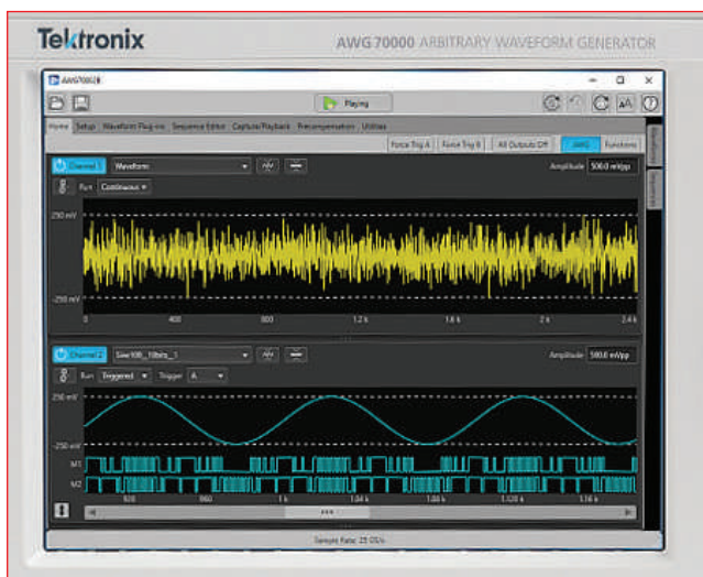
▲ Fig. 1 With 50 GSPS sampling, 20 GHz frequency range and up to 32 GS memory, the Tektronix AWG70001B AWG generates complex waveforms for real-world radar, EW and communications testing.
